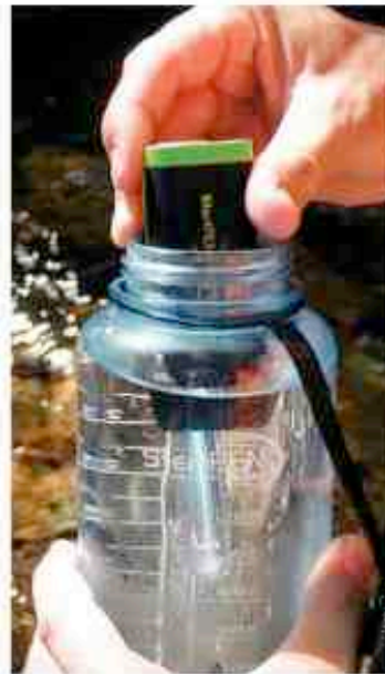
The SteriPEN AdventurerOpti UV water purifier includes an integrated flashlight.
