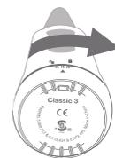
Replace battery cap by aligning cap with open lock icon. Then, rotate cap clockwise until arrow points to closed lock icon.
